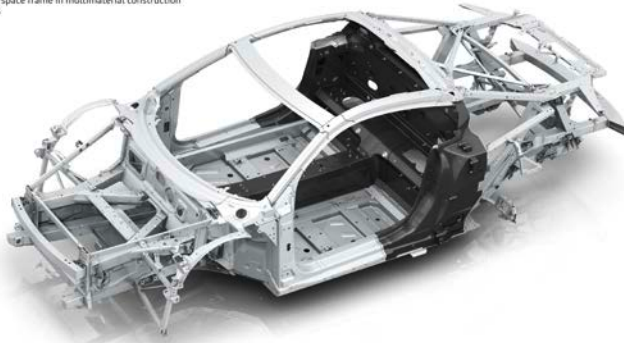
Audi R8 Coupé Audi Space Frame in Multimaterialbauweise Audi space frame in multimaterial construction 07/15
